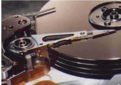
**Figure 2.** Read/write head over the platters [2]
