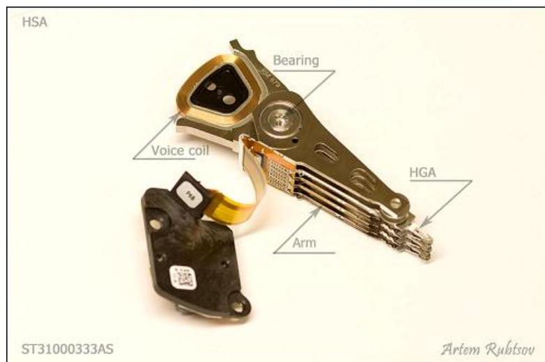
**Figure 3.** Read/write head operating system [2].
